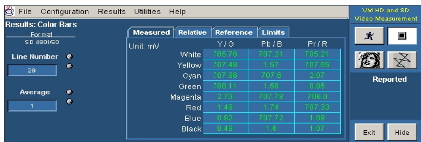
Figure 3-28: Displaying the Color Bars measurement
