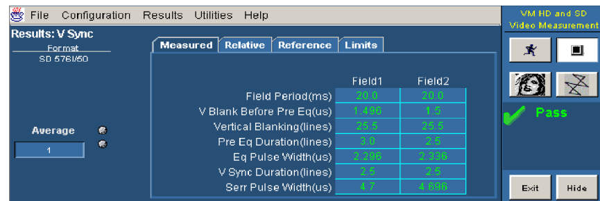
Figure 3-51: Displaying the V Sync measurement for SD Interlaced format
